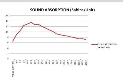
The Tri-Trap© was lab tested at the prestigious Riverbank Acoustical Laboratory and showed to have true effects at 50Hz and below. The Tri-Trap© has been effectively designed to absorb more low end, but also does an excellent job of absorbing the high end, creating smooth sound absorption from 50 Hz to 5000 Hz.
